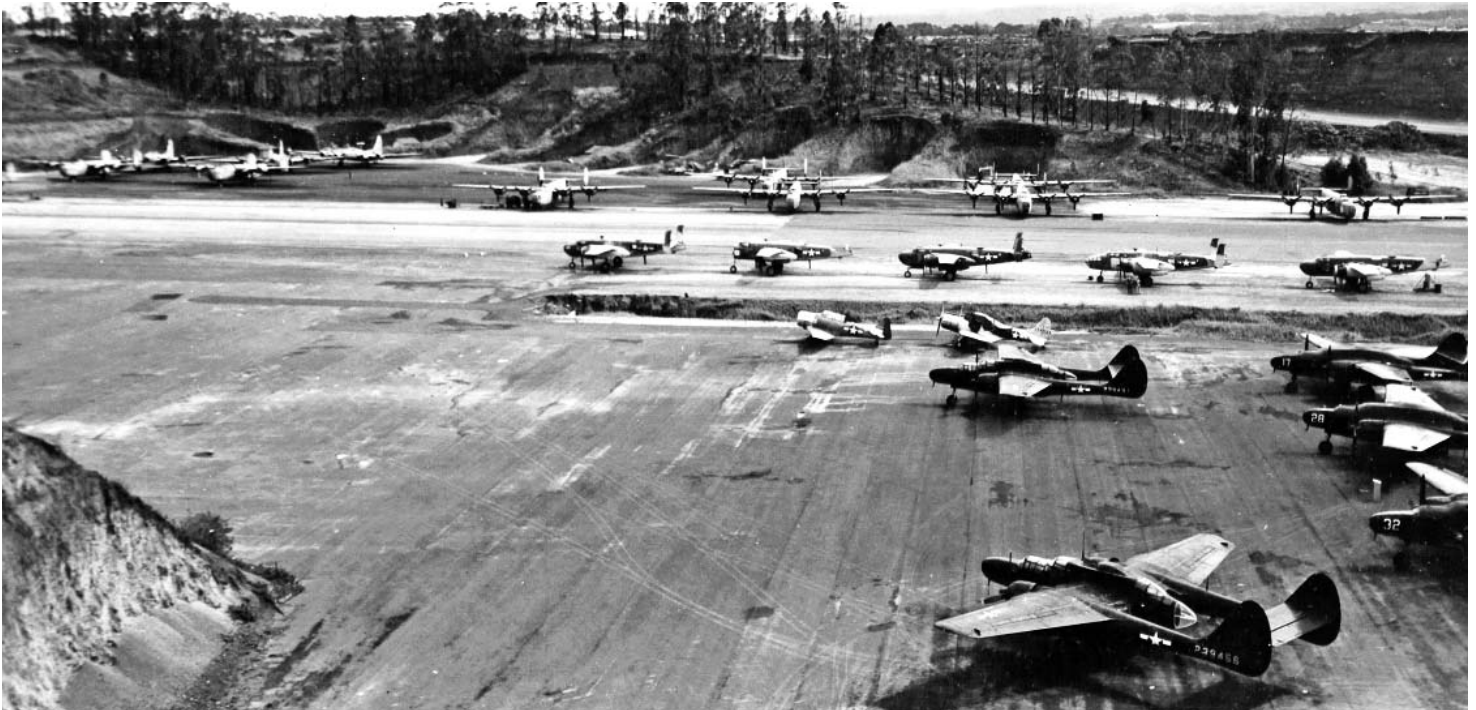
Caption reads: "War weary Northrop P-61s, North American B-25s and Consolidated B-24s rest in the graveyard at Wheeler Field, Oahu, T.H., where they will be stripped for salvage. Note tails removed from the B-25s. April 4, 1945." (Photo from NARA 342FH-3A41110-75056AC, courtesy of footnote™)
